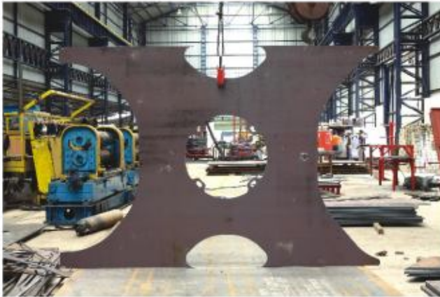
Before Shot Blasting
